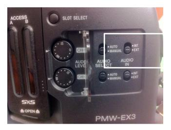
Adjust audio level for CH-1 with the top audio level knob. The corresponding CH 1 switches are set to manual and EXT positions. Remember to use a headset.
